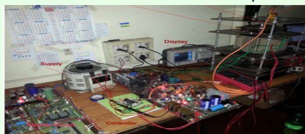
Experimental Setup of the single-axis controlled repulsive-type magnetic bearing
