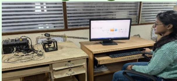
Implementation of a Data Driven Controller on Rotary Servo Flexible Link System interfaced with SIMULINK Real Time Workshop
